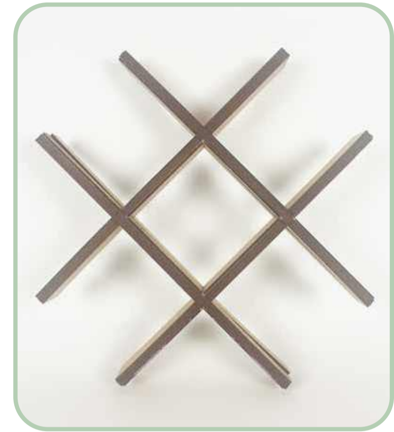
1:20 PHYSICAL MODEL OF A PIECE OF THE MASS TIMBER DIAGRID
